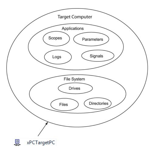
The API object hierarchy derived from the Simulink Real-Time system is shown in this conceptual diagram.
